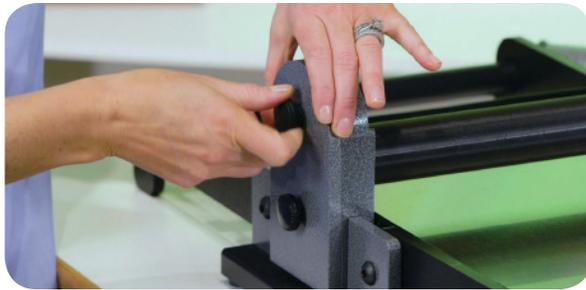
If you have a MARK IV Machine you will need to use a 3/32" hex wrench to remove the two screws.
